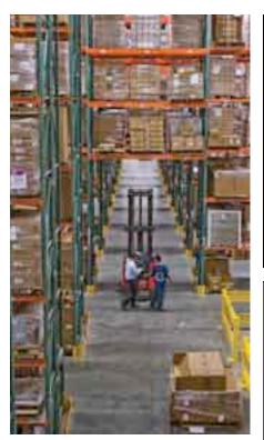
**TALL ORDER** The metal racking system spans up to 40 feet in height at some locations.
